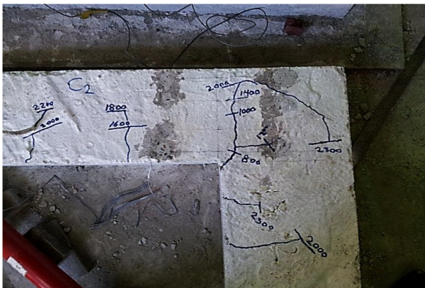
Fig.(3) Crack pattern of the control specimen (C2)
